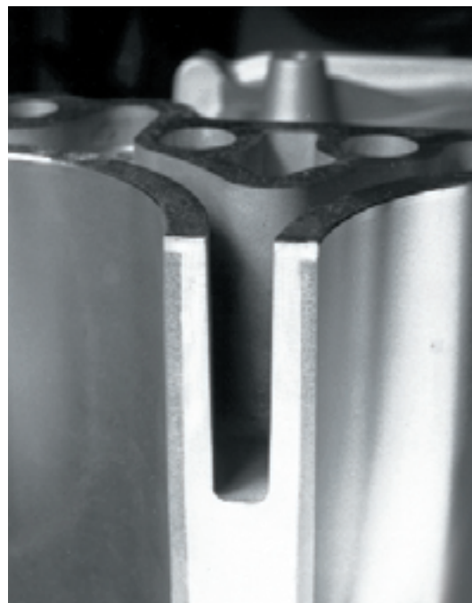
LOKASIL® cylinder bore surface (local silicon enrichment)
